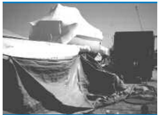
Boat enclosed for plastic media hull blasting.
