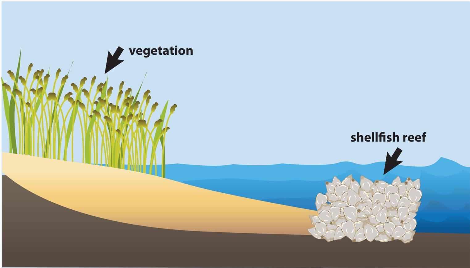
Oyster reefs (see page 5) break up wave energy allowing for sediment deposition and plant life to thrive.
