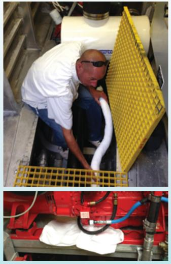
Oil absorbent booms, sheets (bottom), and pads can be kept on your boat to catch leaks under the engine or to contain and remove oil at the surface of the water (back). Bilge socks (top) trap any oily overflow on board, making safe disposal easy. (MASGC/Tara Skelton)
