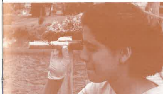
Mausmi Mehta, a student from MIT, measures salinity from a water sample in West Neck Bay, Shelter Island for the Caron/Lonsdale project.
