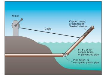
New dry hydrants and strainers should be made of materials (such as copper or galvanized steel) least likely to become fouled by zebra mussels. The intake end of the pipe could be coated with an antifoulant coating such as cuprous oxide paint. The use of such paints may, however, have negative environmental consequences and should not be undertaken without consultation with local environmental officials. Another alternative would be to galvanize the intakes.
