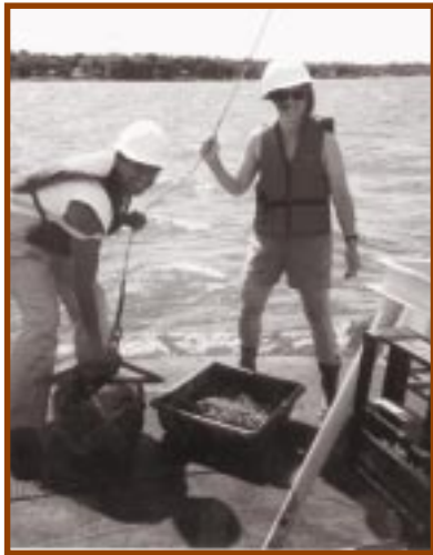
Above photo: (left to right) Chun-Der Li and Josephine Aller realign a VanVeen grab sampler. The sampler's contents, emptied into the pan, will be used to enumerate bottom-dwelling animals and analyze grain size.
