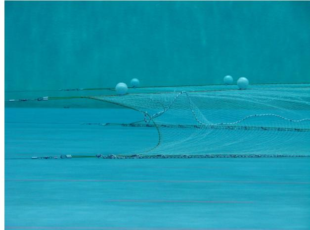
*Lake Ontario scale model trawl being tested in the Memorial University of Newfoundland flume tank, the largest in the world.
